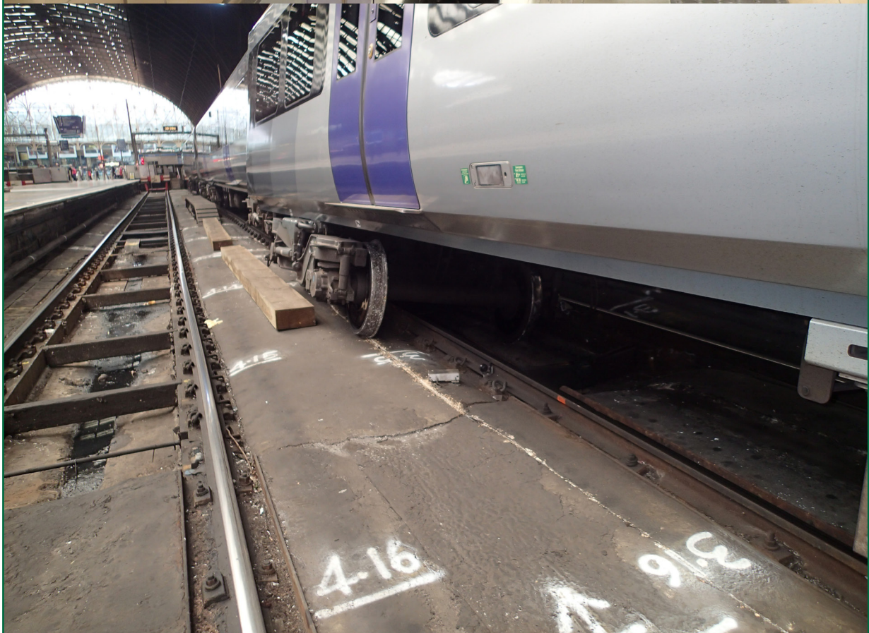
Figure 2: Final resting position of derailed vehicle at Paddington station platform 3
