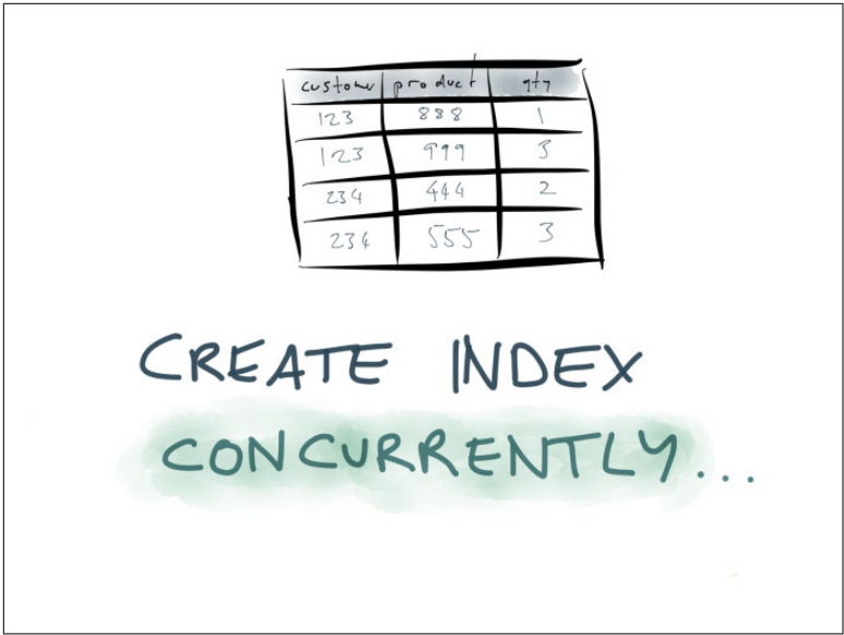
Figure 5-8. The CONCURRENTLY option in PostgreSQL allows an index to be built without locking the base table for writes.
