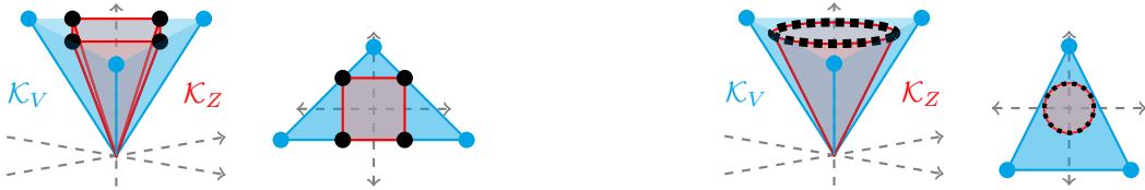
(a) Rows of \mathbf{Z} are extreme rays of the generated “square” cone \mathcal{K}_Z . The square cone can be enclosed by a “triangular” cone \mathcal{K}_V .
