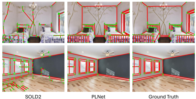
Fig. 6. The line detection comparison between our PLNet (a wireframe parsing method) and SOLD2 (a non-wireframe-parsing method). The red lines are detected line features and the green points are endpoints of lines. Our PLNet aims to detect structural lines while SOLD2 detects more general lines with significant gradients, such as the patterns on the floor and walls.
