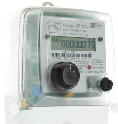
Fig. 1. OneMeter beacon with optical sensor attached to IEC 62056-21 port of electricity meter.
