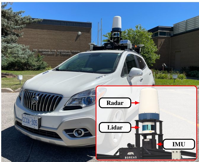
Fig. 10. This figure depicts our data collection platform Boreas which includes a Velodyne Alpha-Prime 128-beam lidar, a Navtech CIR304-H radar, an Applanix GNSS/IMU, and a FLIR Blackfly S camera.
