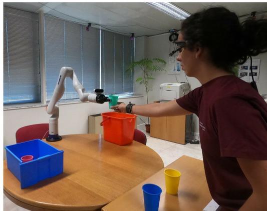
Fig. 1: A human handover of a cup with water to a robotic arm. The robot pours the water into the (orange) bucket and then places the emptied cup into the (blue) drawer. Human is wearing an eye-tracking device, infrared motion tracking markers, and an IMU sensor on the wrist
