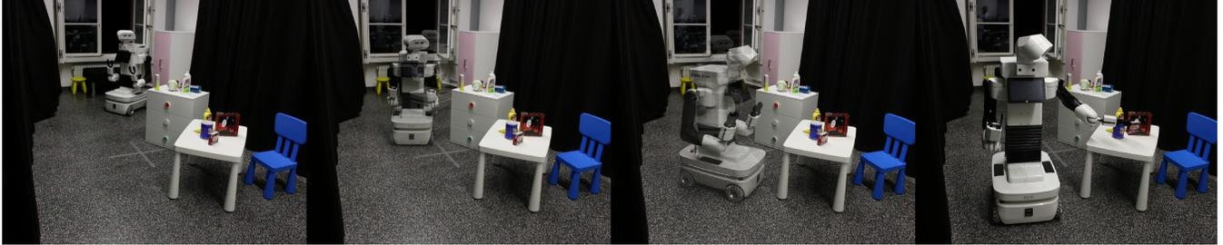
Fig. 1: Real-world execution of our active perception and grasping pipeline. The mobile manipulator robot, equipped with a head-mounted camera, efficiently explores the scene to detect grasps on the target object and effectively performs the grasp by evaluating its executability. Video demonstrations are provided in the supplementary video and the project website: [sites.google.com/view/actpermoma](https://sites.google.com/view/actpermoma).
