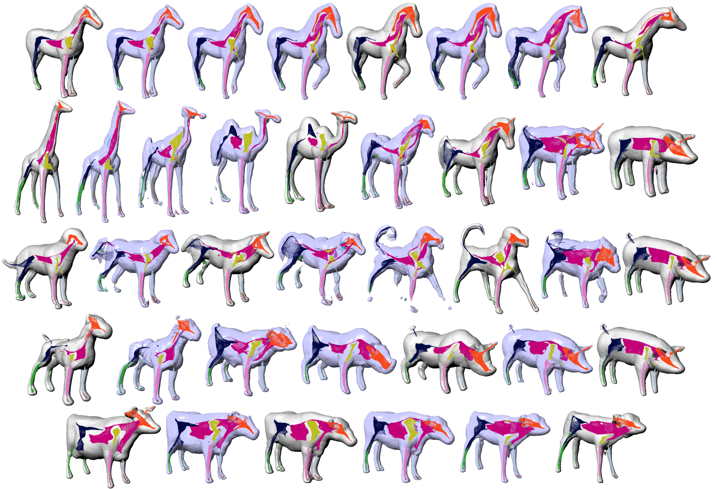
FIGURE 12: Row-wise MARF interpolations in latent space. We illustrate the medial axis by superimposing the medial atom centers associated with each hitting camera ray on top of a Lambertian shading using analytical normals (Eq. 5). We trained this MARF on the COSEG [93] “four-legged” object class, featuring a total of 20 shapes. Gray renders use known auto-decoder latent vectors, while the blue-tinted renders are in-betweens interpolations. Despite the sparse dataset, we find the MARF propose smooth and meaningful in-betweens.
