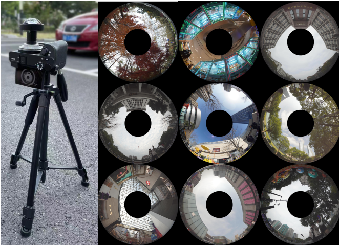
Fig. A.1. The shooting device and sample images of PALHQ. With a well-designed PAL of 11 lenses and a Sony \alpha 6600 camera (on the left), we capture high-quality panoramic images covering various scenes including indoor, natural, urban, campus, and scenic spots (on the right).
