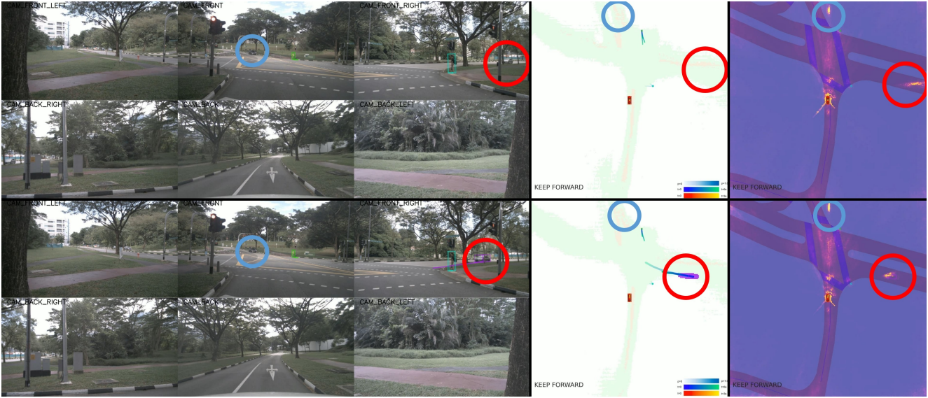
Figure 12. Visualization for planning recovering from perception failures. We show an interesting case where inaccurate results occur in prior modules while the later tasks could still recover. The top row and the down row represent two consecutive frames from the same scenario. The vehicle in the red circle is moving from a far distance toward the intersection at a high speed. It is observed that the tracking module misses it at first, then captures it at the latter frame. The blue circles show a stationary car yielding to the traffic, and it is missed in both frames. Interestingly, both vehicles show strong reactions to the attention masks of the planner, even though they are missed in the prior modules. It means that our planner still pays attention to those critical though missed agents, which is intractable in previous fragmented and non-unified driving systems, and demonstrates the robustness of UniAD.
