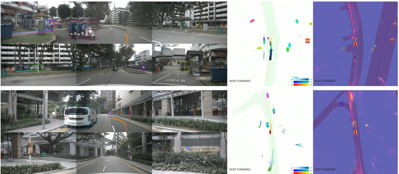
Figure 11. Obstacles avoidance visualization. In these two scenarios, the ego vehicle is changing lanes attentively to avoid the obstacle vehicle. From the attention mask, we can observe that our method focuses on the obstacles as well as the road in the front and back.
