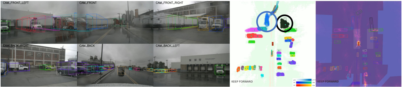
Figure 13. Failure cases 1. Here we present a long-tail scenario, where a large trailer with a white container occupies the entire road. We can observe that our tracking module fails to detect the accurate size of the front trailer and heading angles of vehicles beside the road.
