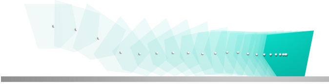
Fig. 6: We drop a polytope-shaped object on flat ground, this simple benchmark scenario highlights the face-to-face contact issue. We quantitatively evaluate the amount of ground penetration and the simulation robustness (Fig. 9).
