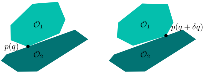
Fig. 5: The contact point between two shape primitives \mathcal{O}_1 and \mathcal{O}_2 can change significantly for arbitrarily small relative pose changes, i.e. the contact location p(q) is a discontinuous function of the configuration q .
