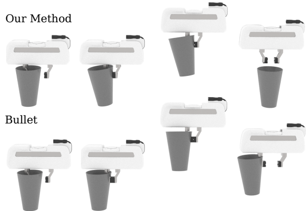
Fig. 3. We control the gripper to pick up a cup and place it at a nearby location. Our simulator can successfully perform the task while Bullet fails due to interpenetrations between the gripper and the cup.
