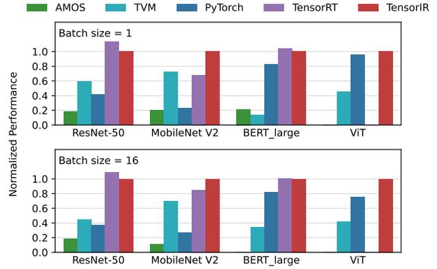
**Figure 12: End-to-End model evaluations on NVIDIA GPU. TensorIR significantly outperforms existing machine learning compilation solutions and achieves similar or better throughputs on popular networks compared with the inference libraries on GPUs. TensorIR get better performance on ViT, an emerging model that TensorRT does not yet support.**
