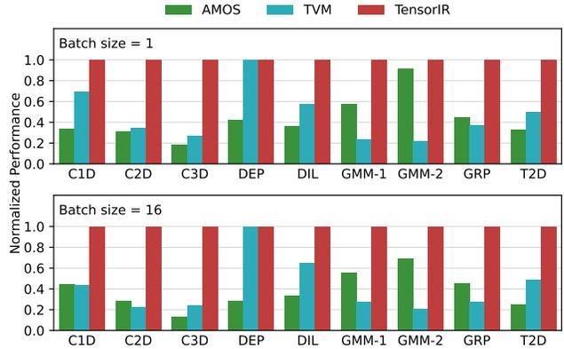
**Figure 10: Single operator comparison to existing machine learning compilers on Nvidia GPU. TensorIR brings up to 7.5x speed across workloads.**
