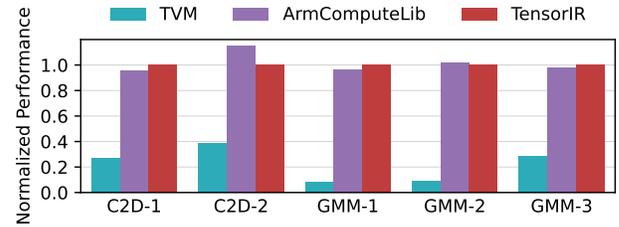
**Figure 13: Single operator evaluations on ARM CPU. TensorIR get up to 12.6x faster than TVM due to the use of native tensor intrinsic acceleration. It also gets to the same level of performance as heavily optimized platform specific library (ArmComputeLib).**
