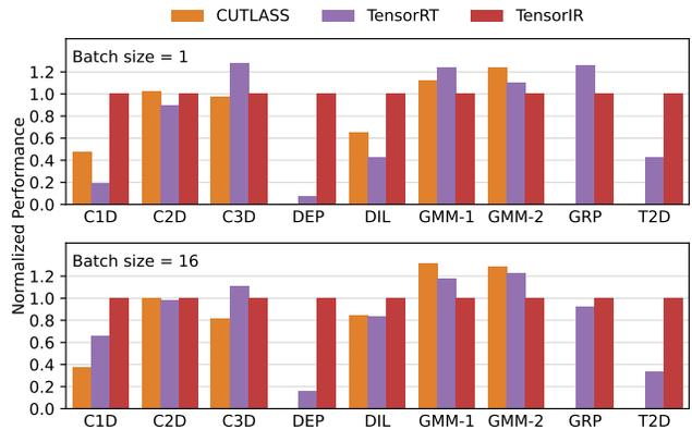
**Figure 11: Single operator comparison to platform-specific libraries. We did not show the numbers of CUTLASS on DEP, GRP, and T2D as the library does not support them. TensorIR outperforms the baselines on C1D, C2D, DEP, T2D, and DIL by up to 13.9x and gets to more than 75% throughput on C3D, GMM, and GRP.**
