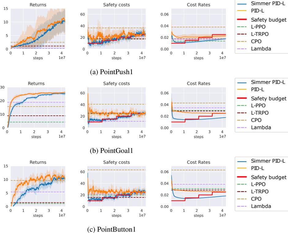
Figure 6: Results for the point robot in the goal, button, and point environments. Simmer PID-L outperforms all baselines in terms of the cost rate, which is a measure of safety during training. At the same time, Simmer PID-L is competitive with PID-L in terms of the returns or safety costs, while significantly outperforming other baselines. The curves are means and shaded areas are variances computed over 5 runs with random seeds.
