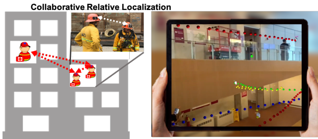
Figure 1: LocAR offers a distributed infrastructure-free relative localization framework that allows multiple mobile users to create a collaborative AR session.
