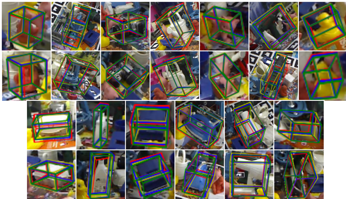
Figure 6. Qualitative results on LINEMOD dataset. Green : the ground truth pose. Red : un-normalized scale prediction. Yellow : normalized scale prediction. Blue : ensemble prediction by averaging the keypoints predicted at both the scales.
