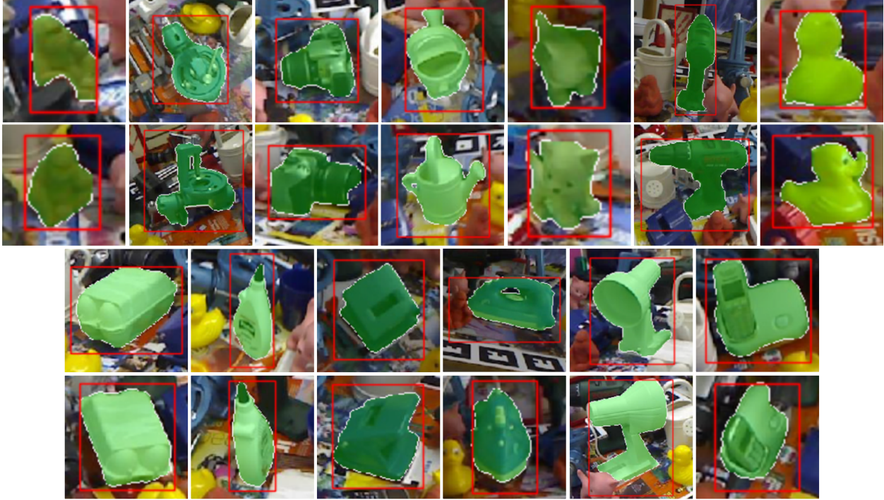
Figure 4. Visualization of given bounding-boxes (red box) and generated pseudo labels (green region) on LINEMOD.
