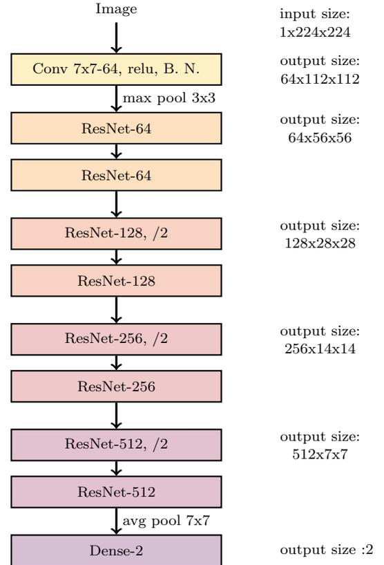
**Figure 8.** Architecture of the ResNet deep compressor. This network compresses the Kaiser-Squires weak lensing map into a two-dimensional summary statistic, which is constructed to be informative with respect to our two unknown cosmological parameters. These informative summaries are evaluated for all the many simulated mock data maps and the single observed data maps to be used for the likelihood-free inference step.
