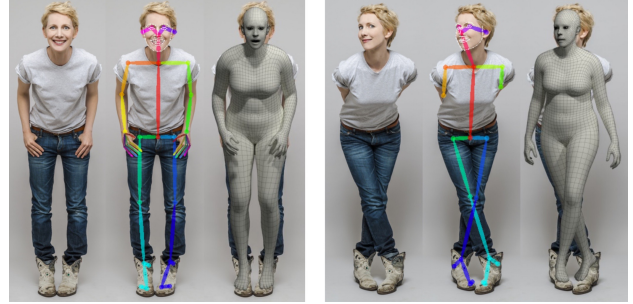
Figure A.4. Failure cases for SMPLify-X with the female SMPL-X for expressive RGB images similar to the ones of Figures 1 and 2 of the main paper. In the left case, 2D keypoints are reasonable, but due to depth ambiguities the torso pose is wrong, while the head shape is under-estimated. In the right case, the arms and hands are occluded and due to lack of constraints the arm and hand pose is wrong. The ordinal depth for feet is estimated wrongly, while similarly to the left case the torso pose and head shape are not estimated correctly. Left : Input RGB image. Middle : Intermediate 2D keypoints from OpenPose. Right : SMPL-X fittings overlaid on the RGB image.
