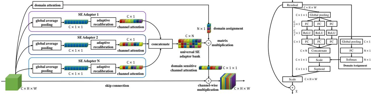
Figure 5. The block diagram (left) and the detailed view (right) of the proposed domain adaptation module.
