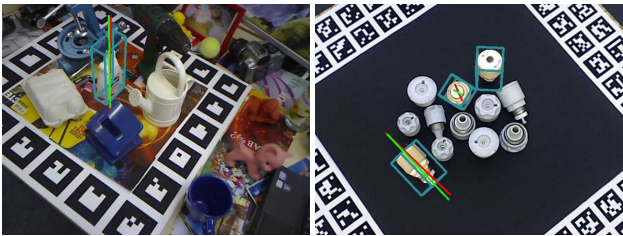
Figure 6: Ambiguity detection. Symmetry axis (green line) estimation. Notice that one screw was classified to be unambiguous ( i.e. no axis), because the ambiguity could be resolved through the texture.
