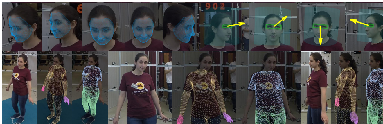
Figure 1: We present a new large dataset of multiview human body expressions for modeling view-specific appearance and geometry. 107 synchronized cameras capture the expressions of 772 distinctive subjects. We focus on five elementary expressions: face (blue), gaze (yellow), hand (pink and purple), body (light orange), and garment including top (light blue) and bottom (light green).
