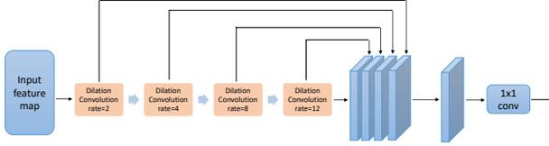
Fig. 4. An illustration of Cascading Dilation Convolutions.
