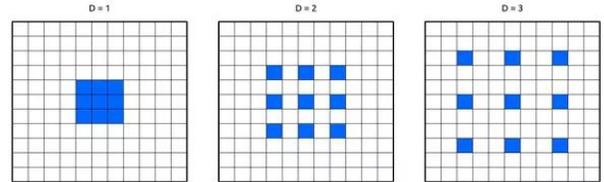
Fig. 3. Dilated convolution: insert zeros into classic convolution to increase the size of receptive fields.
