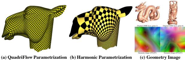
Figure 4: (a) With appropriate method like QuadriFlow, we can get the surface parameterization aligning to shape features with negligible distortions. (b) Harmonic parameterizations leads to high distortion in the scale. (c) Geometry images [15] result in high distortion in the orientation.
