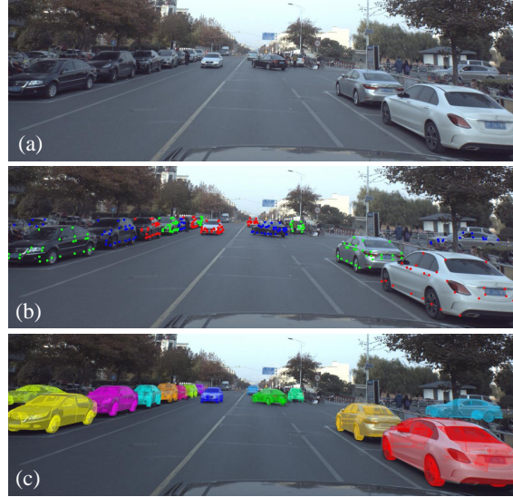
Figure 1: An example of our dataset, where (a) is the input color image, (b) illustrates the labeled 2D keypoints, (c) shows the 3D model fitting result with labeled 2D keypoints.
