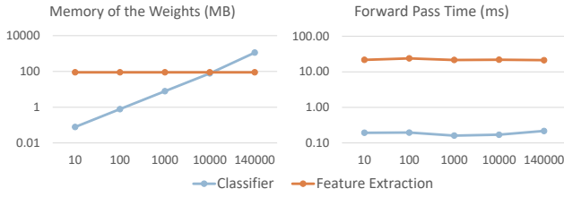
Figure 2: The computational constraints of our model at test time. Orange represents all layers prior to the last fully-connected layer (feature extraction), and blue represents the last fully-connected layer (classifier). With increasing number of classes, the running time barely increases while the memory consumption increases linearly.
