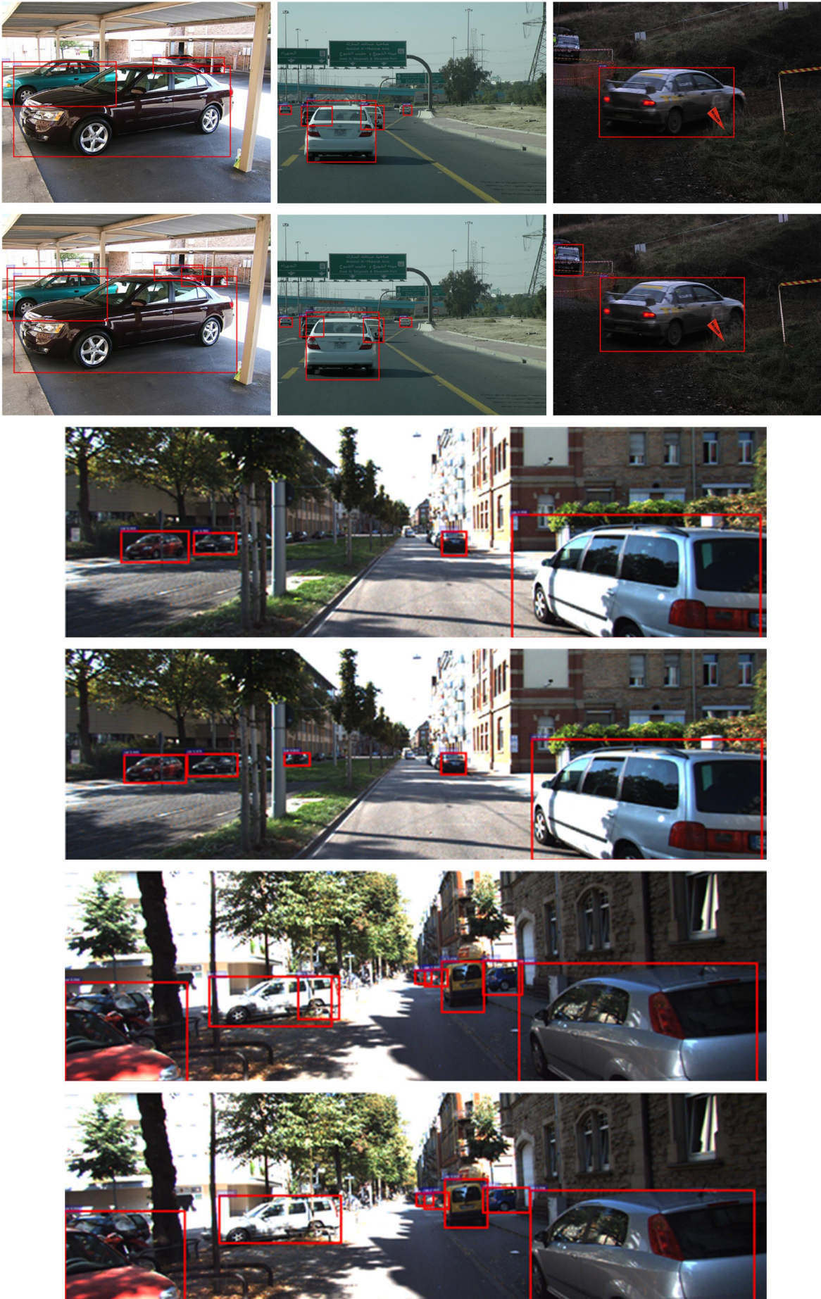
Fig. 9. Examples of object detection results (VGG-16). The upper one of every couple: Objects detected by the model trained purely with the real training set. The lower one of every couple: Objects detected by the model trained with real and virtual datasets.
