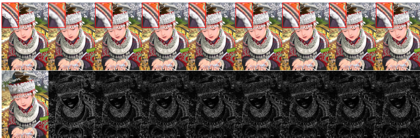
Fig. 4: Comparison of different methods for comic image with scaling factor of 2 (Please refer to the electronic version and zoom in for obvious comparison). Numbers in parenthesis are PSNR, SSIM and SCIELAB error measures, respectively. Left to right: Original, Bicubic (30.46, 0.840, 1.898e4), Zeyde et al. (31.97, 0.887, 1.127e4), GR (31.70, 0.879, 1.198e4), ANR (32.09, 0.889, 1.077e4), NENNLS (31.87, 0.884, 1.159e4), NELLE (32.03, 0.889, 1.099e4), MCcSR (32.23, 0.899, 9.770e3) , ScSR (32.14, 0.893, 1.014e4).
