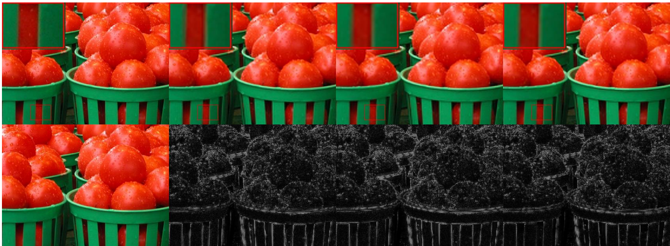
Fig. 12: Visual Images as well as S-CIELAB error maps are shown for a scaling factor of 3. From left to right for each row images correspond to: Original image, applying SR separately on RGB channels (36.26, 0.83, 1.57e4), ScSR (36.13, 0.83, 1.67e4) and MCcSR ( 36.67, 0.85, 1.43e4 ). Numbers in parenthesis are PSNR, SSIM and SCIELAB error measures.
