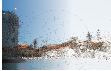
Figure 2: Meshlab visualization, virtual camera with picture overlay. Matching points widely spread in the X-direction of the image.
