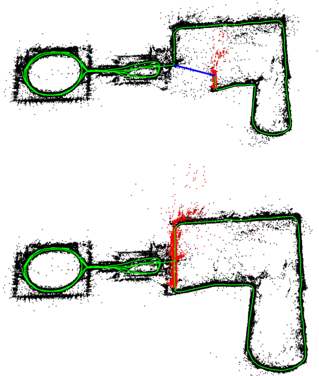
Fig. 5. Map before and after a loop closure in the NewCollege sequence. The loop closure match is drawn in blue, the trajectory in green, and the local map for the tracking at that moment in red. The local map is extended along both sides of the loop after it is closed.
