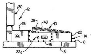
During storage or transport, the keyboard is locked with the housing in a parallel condition to the base housing. When the laptop is used, the keyboard lock can be opened to pop up the keyboard to an ergonomically improved tilted orientation. The structure of the keyboard slopes forwardly and downwardly for comfortable use. Although the keyboard can still be used in a locked flat position.
