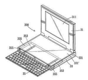
The invention makes a drawer type keyboard concealed within the laptop, which can be pulled or pushed easily according to usage (**Principle-34: Discard and Recover**).
