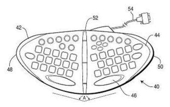
This invention provides a foldable keyboard which consists of two half keyboards consisting of half half keys complementing to each other. When in open position, the first half and the second half make a continuous keyboard. When the keyboard is closed, the first half will be folded over the second half.
