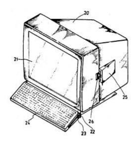
The computer should be space efficient and cheap as well (**Desired result**). The conventional desktop is space hankering. The miniaturisation of a conventional desktop to a laptop makes it expensive (**Contradiction**).
