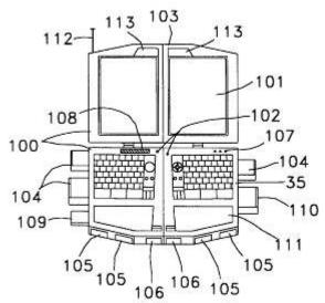
This invention is not confined to only the folding nature of the keyboard. It also has two independent dedicated microprocessors. While one microprocessor use used as a notebook computer, the other microprocessor may be dedicated for video games or a set-top converter box for Internet access through cable TV.
