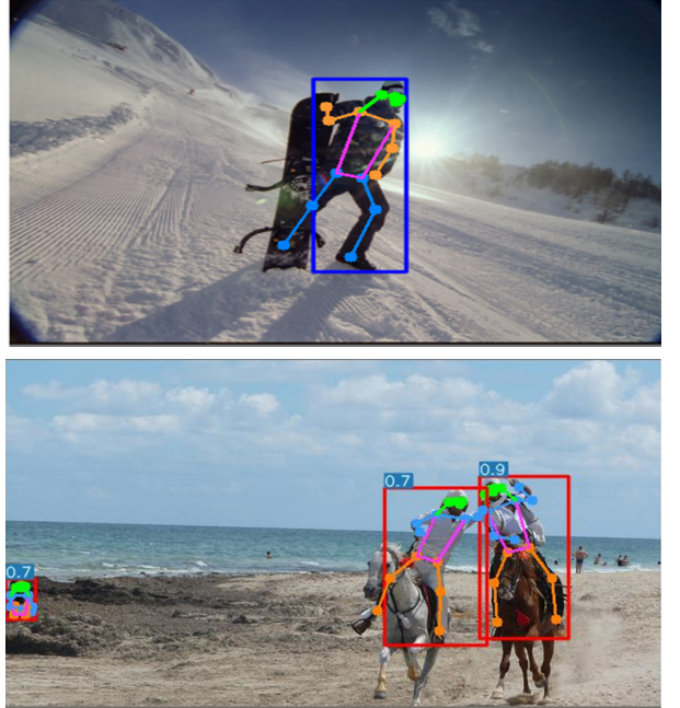
Figure 3. Tackling challenges of top-down approaches. Top: YOLO-pose correctly predicts occluded keypoint lying outside the bounding box. Bottom: For the person in the middle, the box detection is not exact. However, that doesn't constrain the keypoint for the right ankle to go wrong. It's predicted outside the box. Top-down approaches would have missed the keypoint for the right ankle completely.
