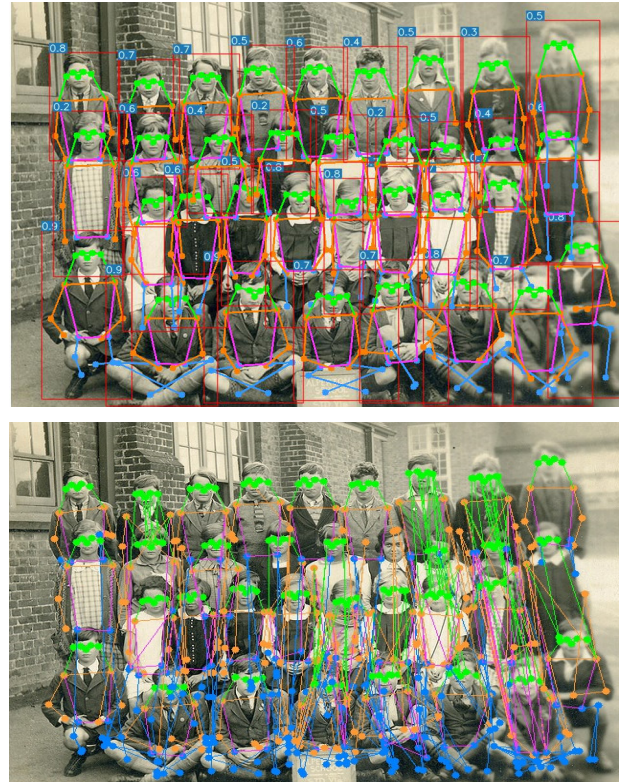
Figure 1. Qualitative result on a crowded COCO val2017 sample image. Top: Output from yolov5m6-pose shows the robustness of our approach. Keypoints of one person is never mistaken with another because of inherent grouping. Bottom: Output from HigherHRNetW32 showing how easily the grouping algorithm fails even when the keypoint locations are mostly correct. Bottom-up approaches are prone to such grouping errors in crowded scenes.
