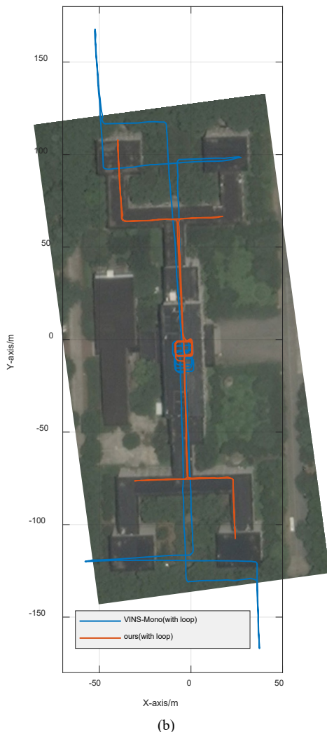
Fig. 7. Path of floor-scale pose estimation (the robot starts from the origin along the positive direction of the X axis, and (b) Projection and alignment of the satellite map of the experimental area to the path map in true scale. The satellite map is taken from Bing.com)
