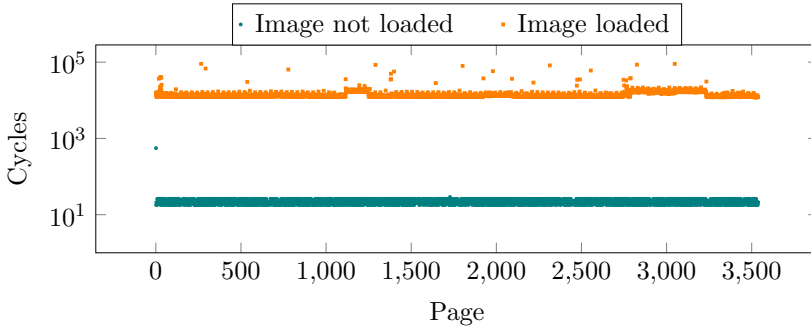
Figure 6.2.: Timings measured in native code on a Linux KVM virtual machine under high CPU load. The graph shows write-access times on an array containing an image file.
