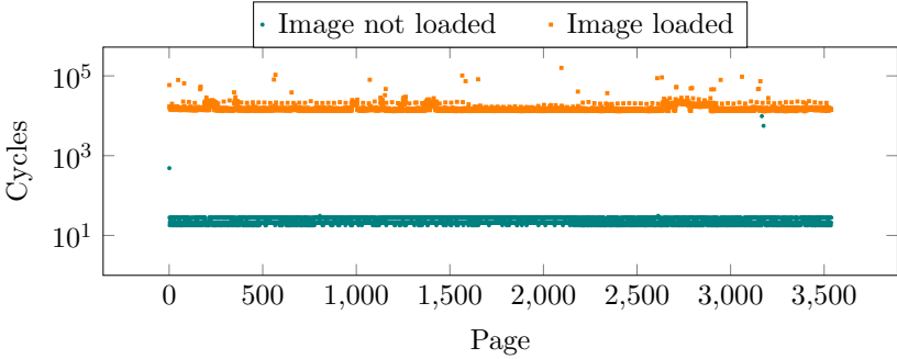
Figure 6.1.: Timings measured in native code on an otherwise idle Linux KVM virtual machine. The graph shows write-access times on an array containing an image file.
