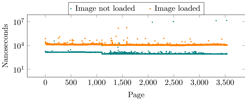
Figure 6.4.: Timings measured in JavaScript on a Linux KVM virtual machine under high CPU load. The graph shows write-access times on an array containing an image file.
