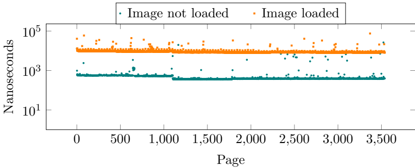
Figure 6.3.: Timings measured in JavaScript on an otherwise idle Linux KVM virtual machine. The graph shows write-access times on an array containing an image file.
