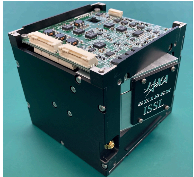
Fig. 1. AOCS module collaboratively developed by the University of Tokyo and Seiren, and JAXA. 5)
