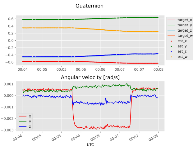
Fig. 12. Target attitude and estimated attitude during the mission operation.
