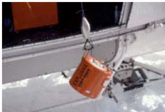
Figure 3. The “carica Vassale” to manage artificial avalanche release with explosives using helicopter (Vassale et al., 2004).
