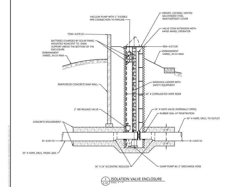
HINGED, LOCKING, VENTED GALVANIZED STEEL, WEATHERTIGHT COVER - BATTERIES (CHARGED BY SOLAR PANEL MANHOLE LADDER WITH MOUNTED ADJACENT TO VALVE ENCLOSURE), SUPPORT ABOVE THE BOTTOM OF THE ENCLOSURE SAFETY EQUIPMENT -CONTROL PANEL 60" ¢ CORRUGATED HDPE RISER
