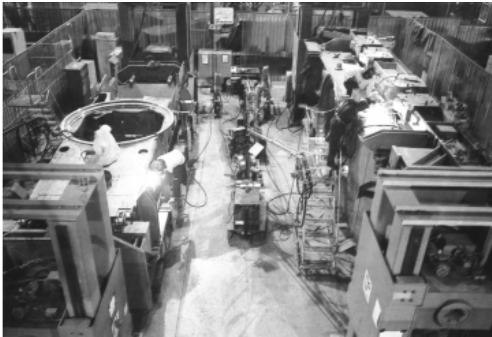
Egyptian workers perform welding operations on two M1A1 tank hulls. Under this coproduction program, all operations necessary to complete the vehicles are performed by trained Egyptian tank plant workers.
