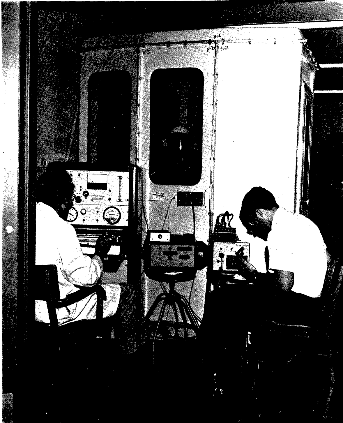
Figure 1. USAFSAM di-2-ethylhexyl phthalate respirator quantitative fit test instrument.
