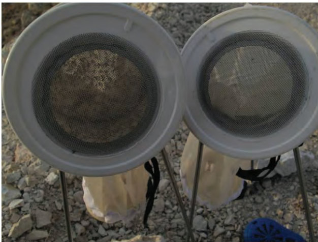
Figure 4. Sand flies in collection cups for traps without a metofluthrin device (right) and with a device (left).
