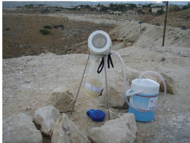
Figure 2. Suction traps were operated in an updraft configuration and suspended in a vertical position by a tripod attached to rocks to prevent it from blowing over in strong winds. \text{CO}_2 from a thermos flask containing dry ice was vented at the trap entrance. A fan vaporizer device emanating metofluthrin was either placed directly below the trap entrance (shown) or clipped onto the side of the trap (not shown).
