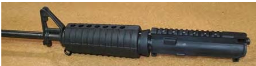
Figure 9. M4 upper receiver with Picatinny rail. The “Picatinny Rail” is defined from a military standard, specifically MIL-STD-1913 (AR) which was adopted on February 3, 1995. This document specified exactly what the dimensions and tolerances were for any mounting systems that were to be submitted for acceptance by the military. The term “Picatinny” comes from the place of origin for this system, the Picatinny Arsenal located in New Jersey. Source: Photograph by author.
