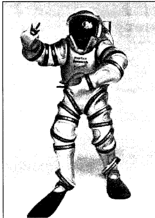
Figure 23: EXOSUIT, prototype atmospheric diving suit. (Courtesy of Nuytco Research Ltd.)
