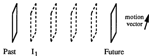
Figure 9: Motion compensated interpolation.
