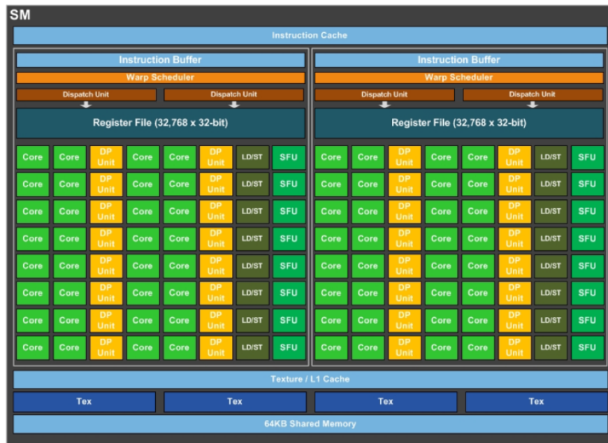
(b) Constituents of a Streaming Multiprocessor (11; 1).
