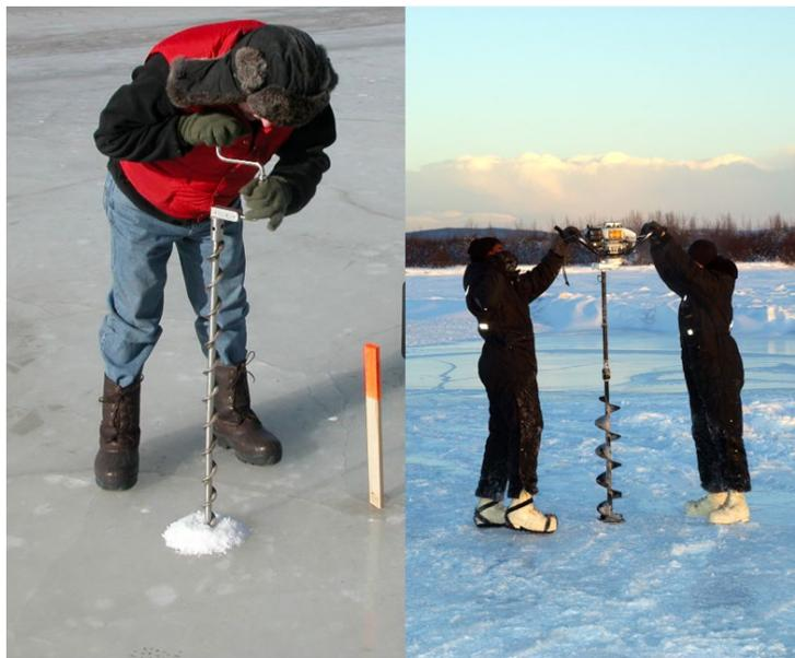
Figure 6.1 Hand operated and gas-powered augers.
