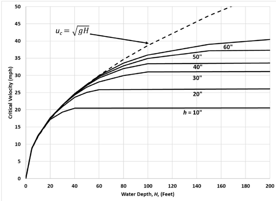
Figure 3.2 Critical velocity as a function of water depth and ice thickness (Nevel 1970). In this figure,  $u_c$  = the critical velocity;  $g$  = gravity;  $H$  = water depth; and  $h$  = the ice thickness.
