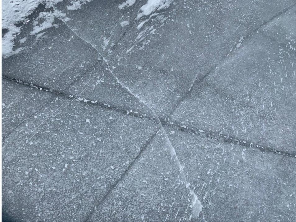
Figure 9.1 Examples of ice cover cracks. A shallow dry crack and refrozen wet cracks are shown.
