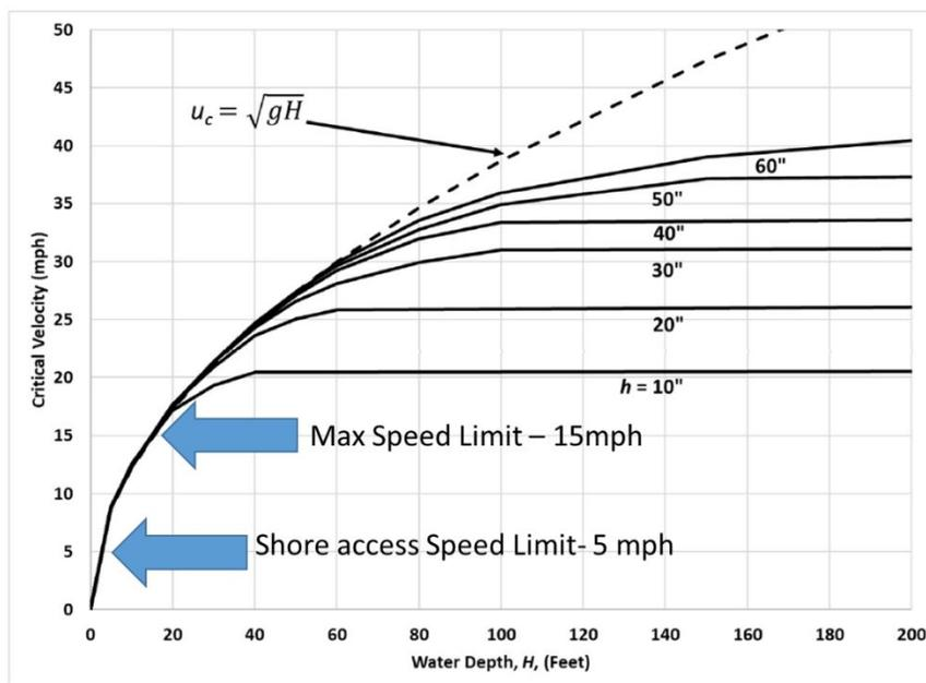
Figure 8.1 Critical Wave Speed as a function of water depth,  $H$ , and ice thickness,  $h$ .
