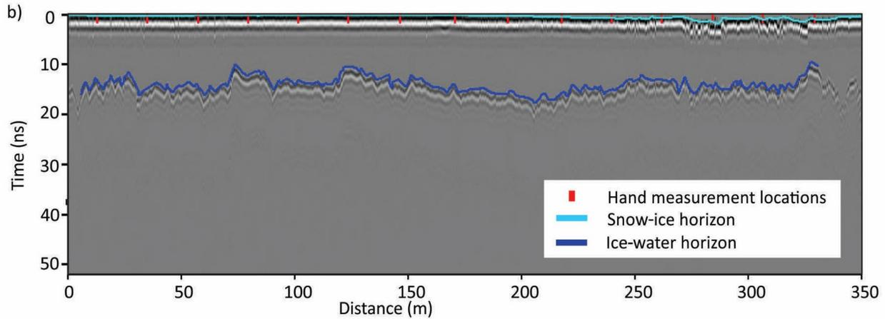
Figure 6.4 Examples of GPR surveying on the Delta River (a) and Yukon River (b) in Alaska. Top panel (a) shows the annotated “Image” (Radargram) of the subsurface. on the Delta River, Alaska. Bottom panel (b) shows GPR measurements on the ice road across the Yukon River near Tanana (Richards et al., 2022).
