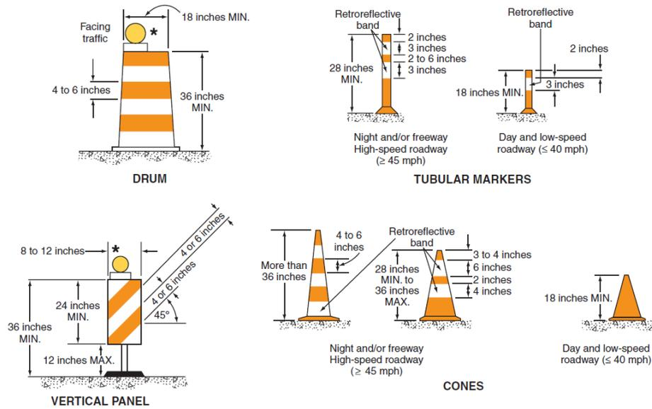
Figure B. 7 Channelizing Devices
