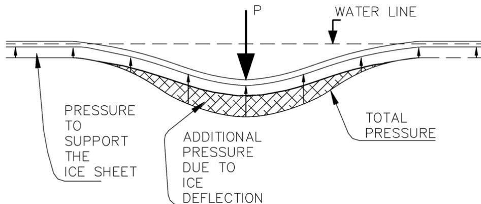
Figure 3.1 Cross section of the deflection bowl created by a point load on the ice (not to scale).
