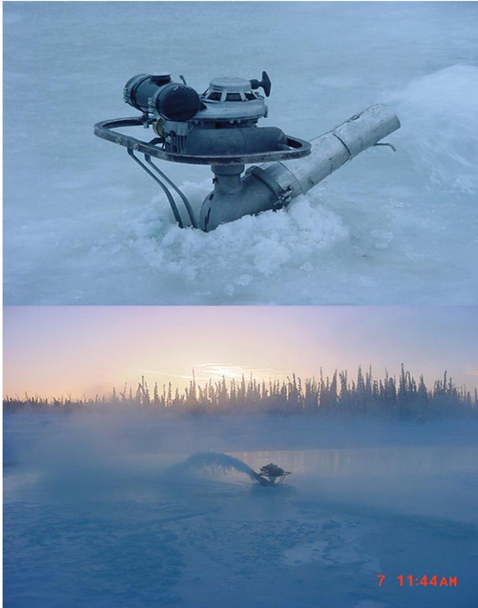
Figure 6.7 Example of pumps for flooding ice surface
