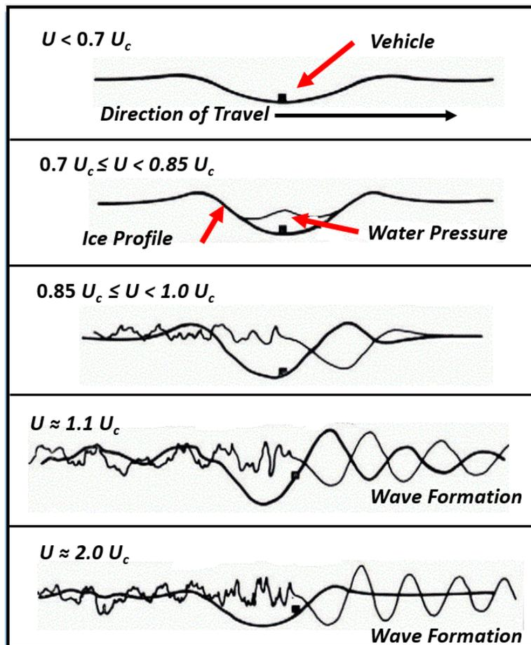
Figure 8.2 Stages of Ice Cover Deflection as a function of the Vehicle speed relative to the Critical Speed.
