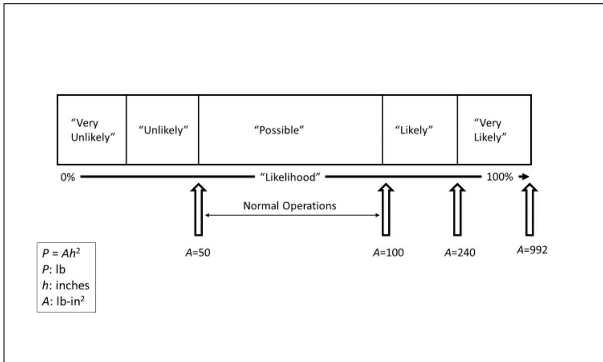
Figure 3.4 Characterizing Failure Risk (Adapted from Hayley and Proskin 2008)
