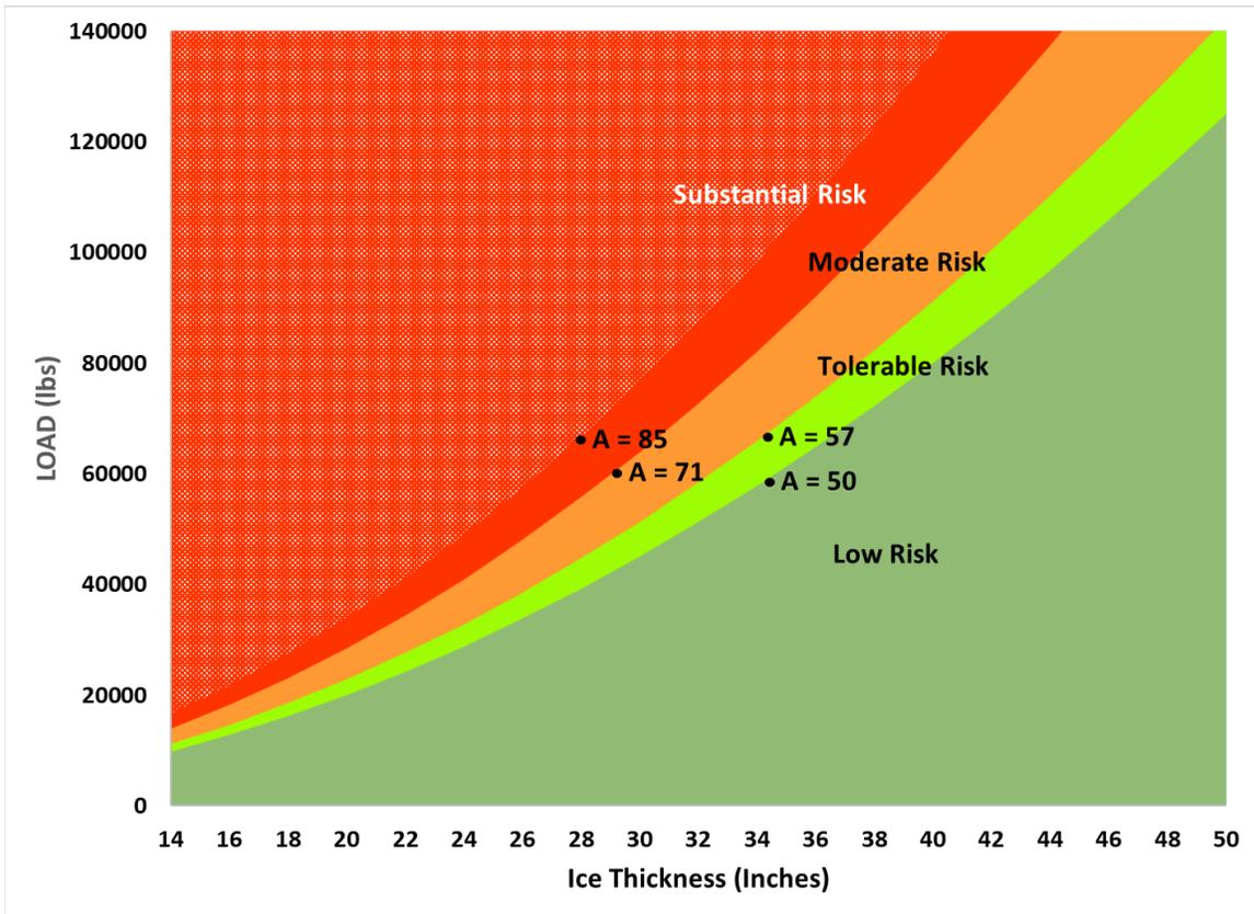
Figure 5.2 Allowable Loads in Pounds for Effective Ice Thickness and A Values
