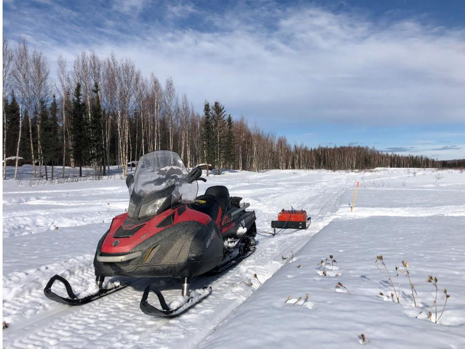
Figure 6.3 Photo of GPR system pulled by snowmachine (Photo credit T. Sullivan).
