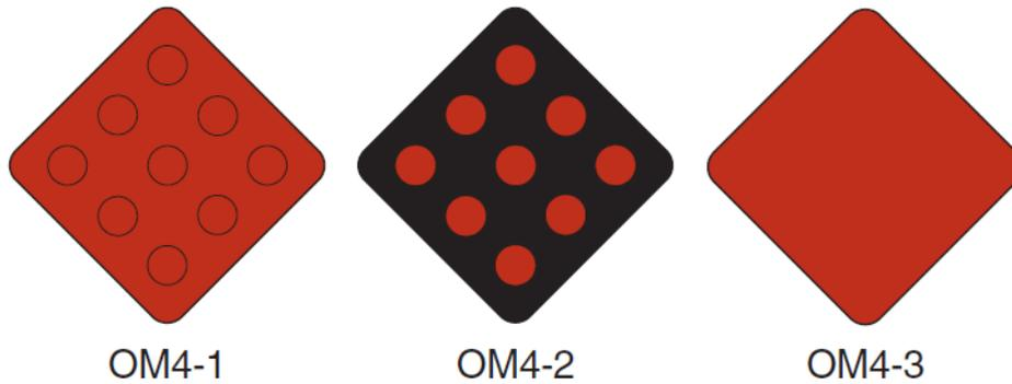
Figure B.6 End of Roadway (Example. MUTCD pg. 536)
