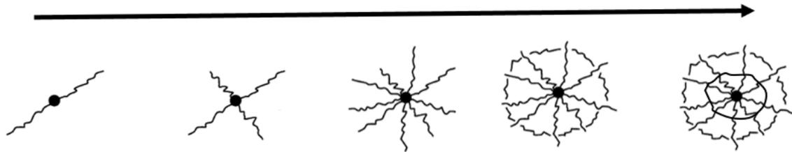
Figure 3.3 Steps leading to ice cover collapse (Ashton (1986) with changes)
