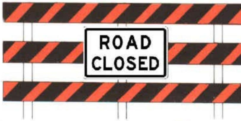
Figure 10.1 Ice Road closure sign mounted on barricade (Saskatchewan Ministry of Highways and Infrastructure 2009)
