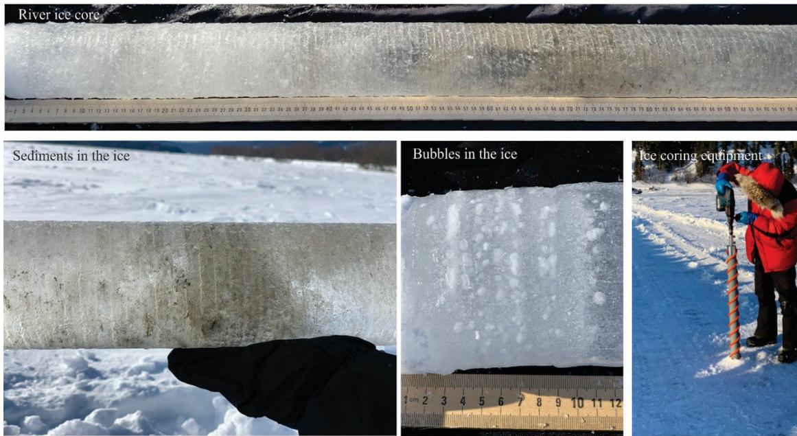
Figure 6.2 Photos showing river ice cores and coring equipment.
