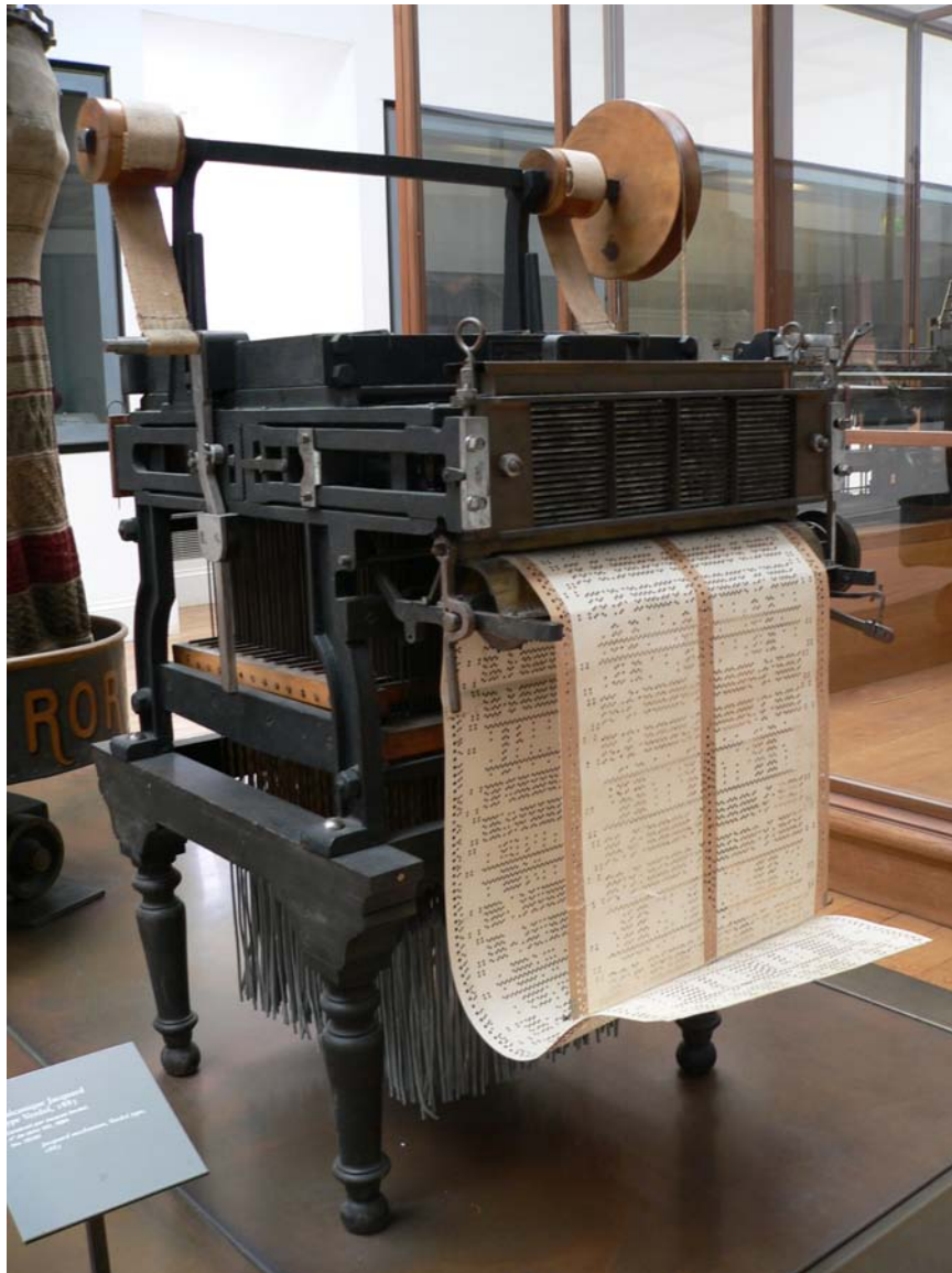
Figure 2.13: Reconstruction of a Jacquard loom.
