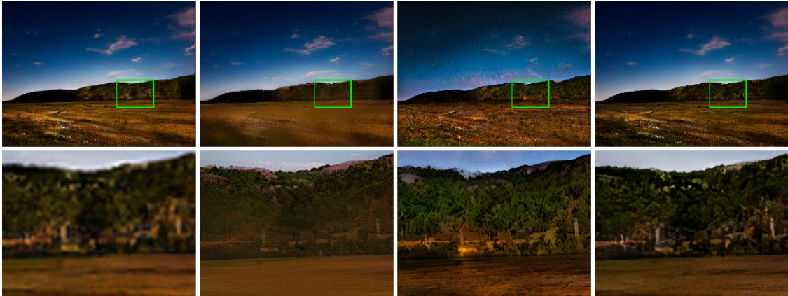
(b) The guided filtering (second column) fails in highly detailed regions, resulting in blurry artifacts.
