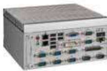
ITA-1711 Intel® Celeron™ J1900 Fanless Compact System with Multiple COM Ports and Dual Displays
