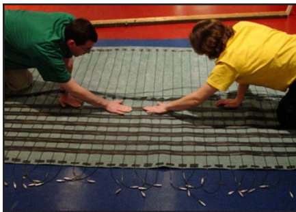
Figure 10.2. Rewiring the carpet with piezoelectric wires. [Photo by Stephanie Hunt].
