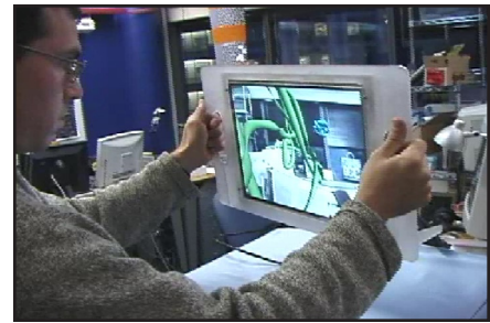
Figure 8.7. Moving the viewscreen around causes the forms to react as if they were exactly where they were placed in the room.
