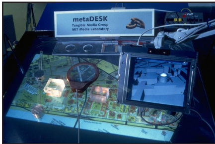
Figure 6.1. Brygg Ullmer's metaDESK uses a variety of physical tools and metaphors to allow users to interact with geographical data.
