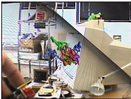
Figure 8.6. In object placement mode, the user can throw the object into the space of the room.
