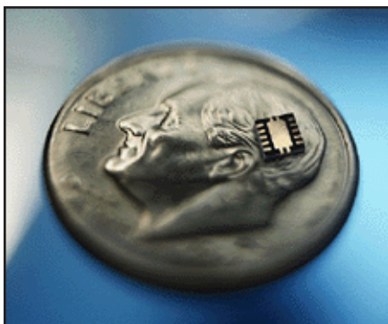
Figure 2.6. Cygnal proudly offers us the C8051xxx microcontroller family. Good luck soldering that one. [ http://www.cygnal.com/ ]
