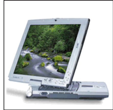
Figure 14.1. Some laptops now allow their screens to be flipped and folded down to make the machine into a tablet controlled with a stylus. This opens up a whole variety of spatial interactions.
