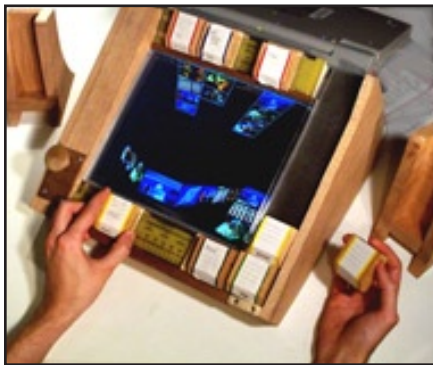
Figure 6.2. Brygg Ullmer's mediaBlocks lets users store and manipulate media clips as if they were stored in wooden blocks.
