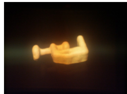
Figure 14.2. An image of a vice as seen on the new 3D display from the Spatial Imaging Group at the MIT Media Lab. (The vice was scanned with EyeBox.)
