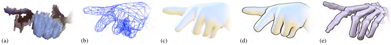
Figure 4: The ShadowHands visualization process: Data from the depth sensor (a) is processed by our hand tracker, producing a coarse 3D hand model (b). We then smooth the model using subdivision, shade it with image-based lighting (c), and add black outlines (d). Additionally, our hand pose information allows us to provide alternate stylized visualizations (e).
